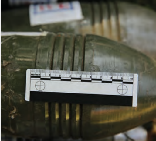
Image 5 Gas-check bands on a 120 mm mortar round manufactured by IS forces Gogjali, Mosul, November 2016
